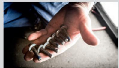
Also very important are the little things, like flywheel bolts. The ones pictured here are for dummy purposes, and couldn't be used to install this flywheel, meaning special bolts needed to be sourced. Ensure you use high-quality flywheel bolts and that they are torqued to the correct specifications.
