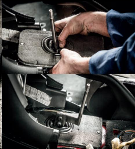
To keep noise and harshness out of the cabin, the boys made up a custom gear surround. Made from a fibreglass plate covered in Dynamat, it includes a generic rubber boot to grip the gearstick, minimizing any unwanted noise that may reach the cabin from beneath the car.
